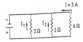
3. Given three resistors, (2 ohms, 3 ohms, and 6 ohms, arranged in parallel with an ideal emf. The directions of the currents in the resistors are shown. The current is 3 amperes in the 6 ohm resistor.
