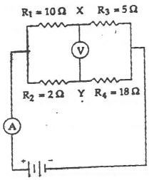
19. Given four resistors joined in two parallel branches as shown. The voltmeter, V, reads 8.5 volts with point Y the plus or higher end. The current in the 2 ohm resistor is A.
