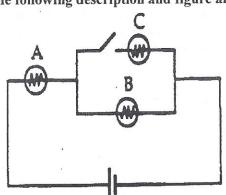
7. Given three identical light bulbs connected with a switch and ideal emf as shown.
