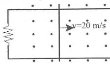
15, 16 Given a wire sliding to the right at a constant speed of 20 m/s. The wire lays across a pair of horizontal frictionless wires serving as "tracks" which are separated by 0.20 m. The wire is moving perpendicular to a vertical constant magnetic field of 2.5 Tesla pointing upward perpendicular to the page. All of the apparatus is in the magnetic field. The resistor in the circuit to the left is 10.0 ohms
